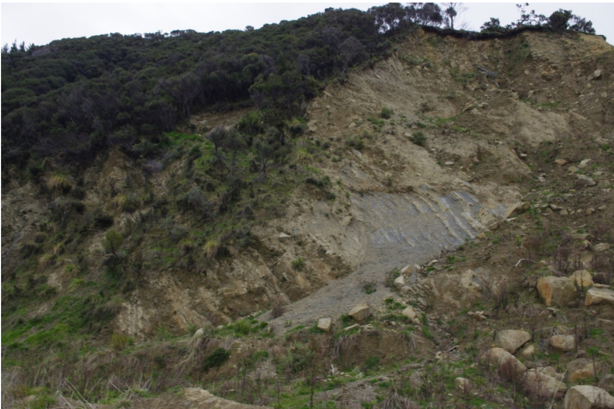
Exposed rockmass on southern side of landslide area acting as side release zone.
